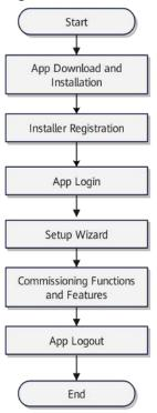
Figure 6-2 Commissioning process on the FusionSolar app
