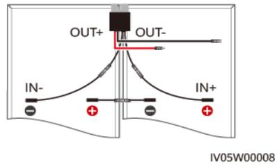
**Step 2** Connect the positive probe of the multimeter to the positive output terminal of the optimizer and the negative probe to the negative output terminal to check the output voltage of the optimizer.
