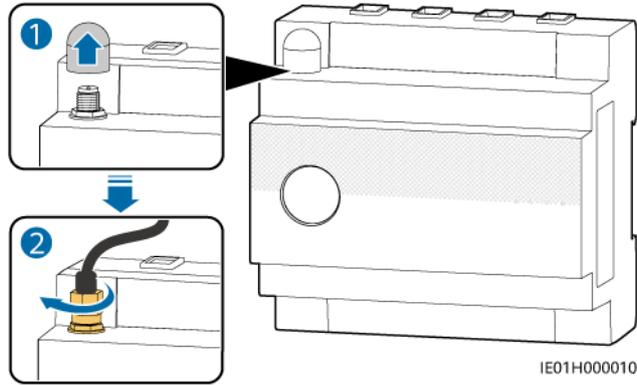
**Step 3** Select an appropriate position and attach the external antenna by magnet.
