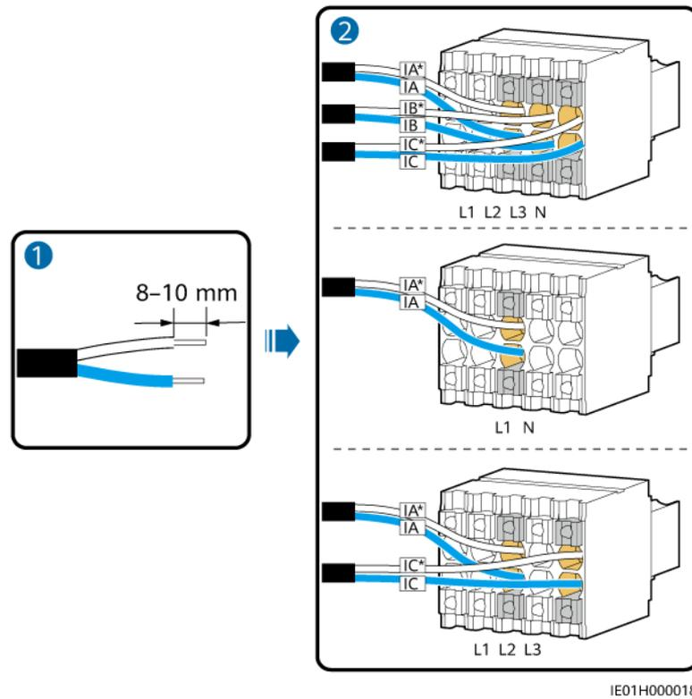
**Step 2** Open the protective cover of the cable fixing screw, insert the AC power cable into the AC input port, and tighten the screw.
