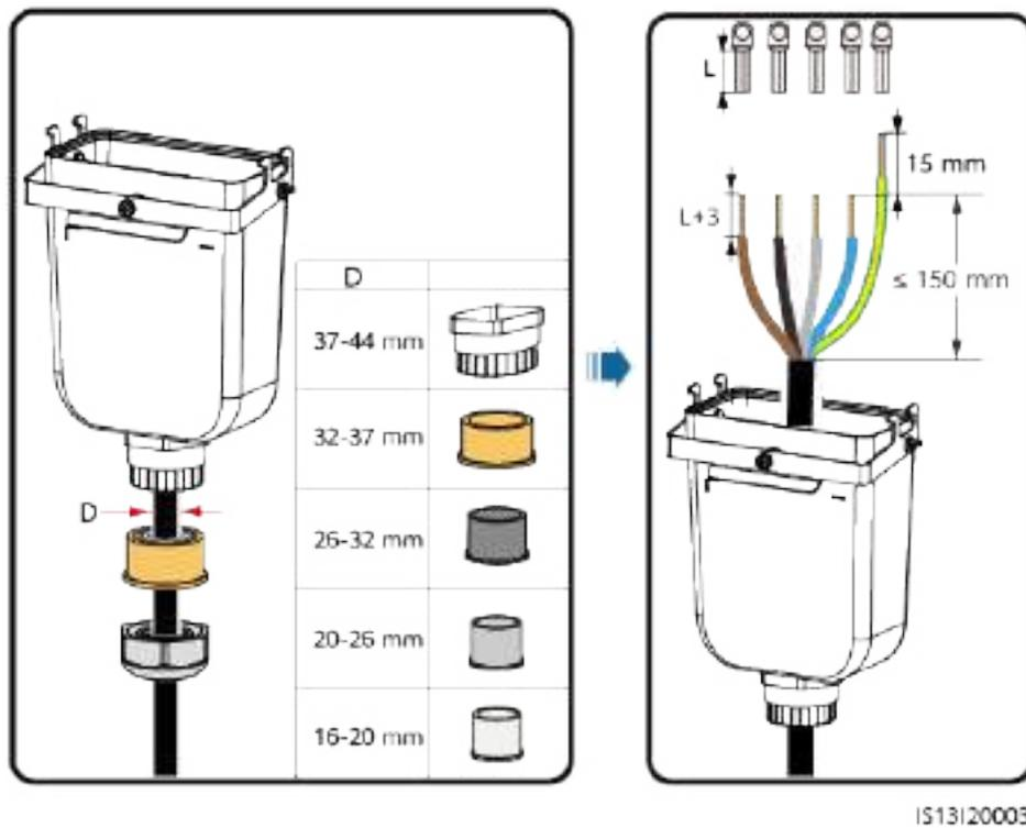
**Figure 5-7** Five-core cable (L1, L2, L3, N, and PE)
