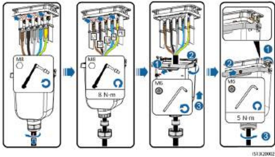
**Figure 5-8** Four-core cable (L1, L2, L3, and PE)
