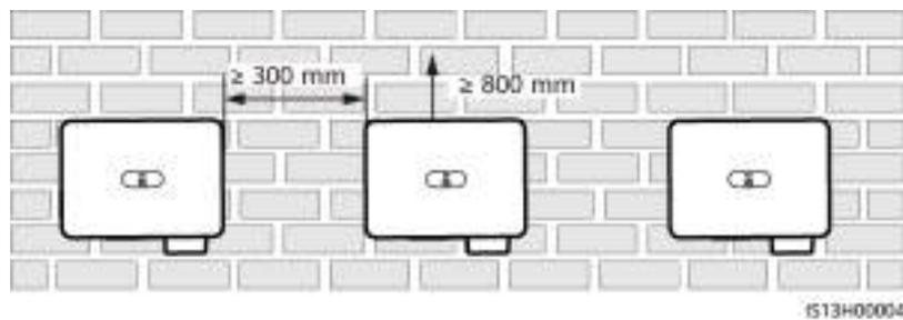
**Figure 4-4** Two-layer triangle installation (not recommended)
