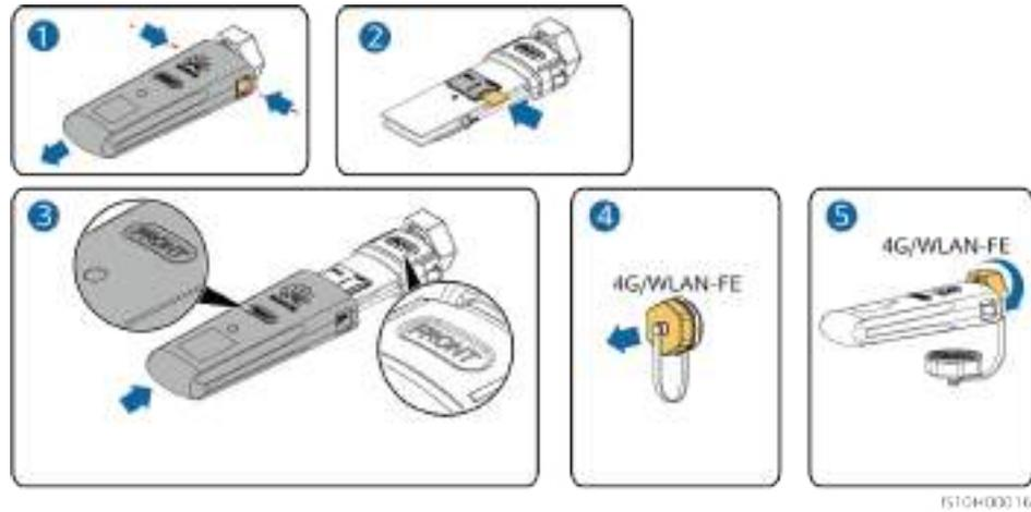
**Figure 5-15** Installing the 4G Smart Dongle (SDongleB-06)
