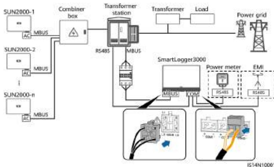
Figure 5-23 MBUS communication (C&I scenario in China)
