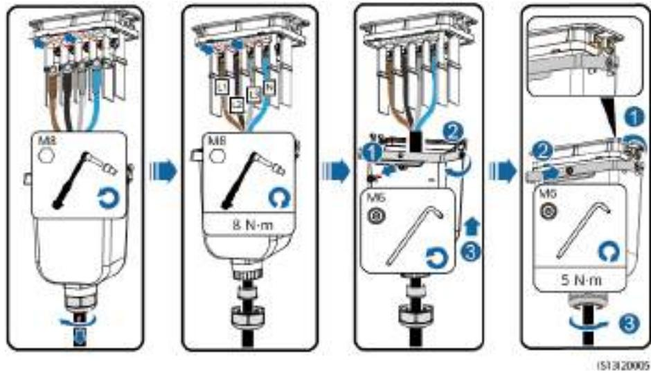
**Figure 5-10** Three-core cable (L1, L2, and L3)
