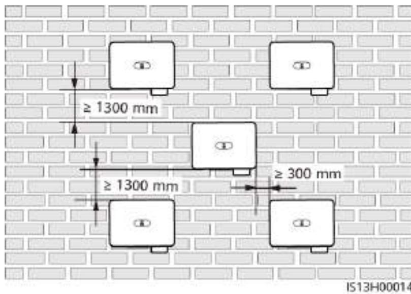
**Figure 4-6** Stacked installation on a wall (not recommended)
