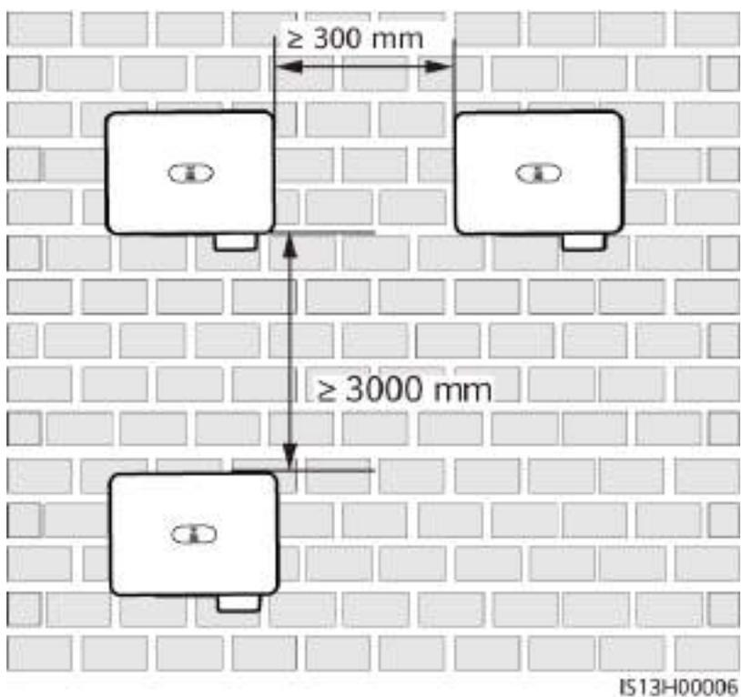
**Figure 4-7** Stacked installation on supports (recommended)
