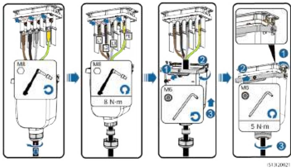
**Figure 5-9** Four-core cable (L1, L2, L3, and N)
