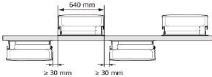
**Figure 4-9** Back-to-back installation on supports (not recommended)
