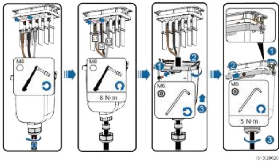
Figure 5-11 Wiring requirements
