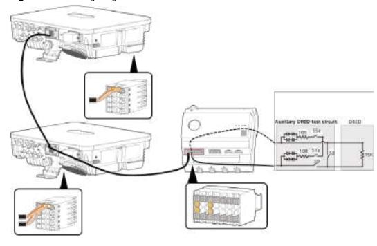
Figure 7-10 Wiring diagram for the DRM function
