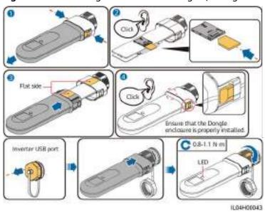
Figure 5-38 Installing anti-theft components for the Smart Dongle
