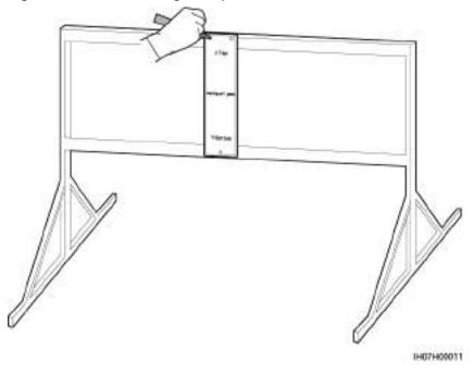
Figure 4-11 Determining hole positions
