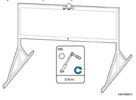
Figure 4-13 Securing the mounting bracket
