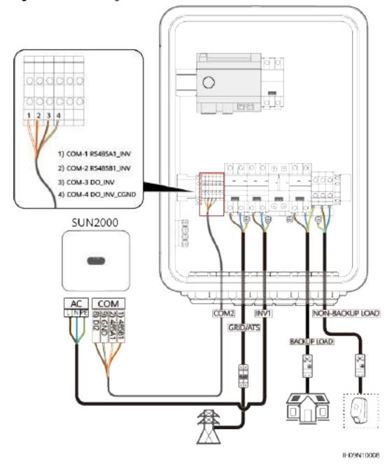
Figure 5-25 Connecting cables to the SmartGuard
