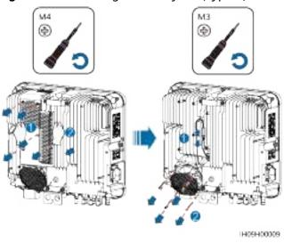
Figure 8-2 Removing the faulty fan(Type 2)
