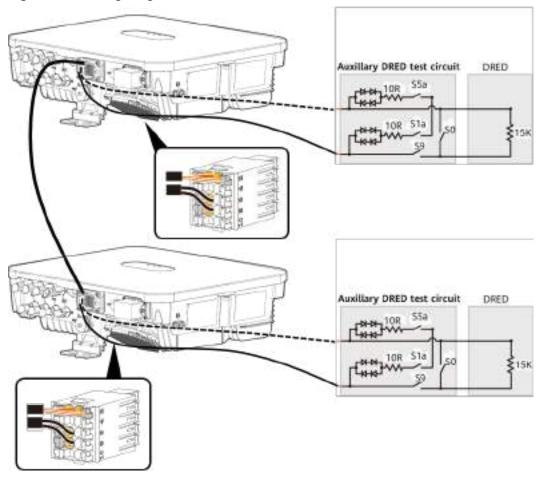
Figure 7-4 Wiring diagram for the DRM function
