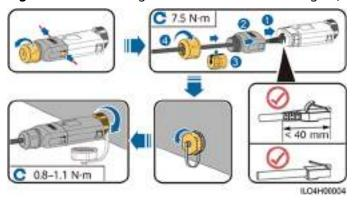
Figure 5-36 Installing anti-theft components for the Smart Dongle
