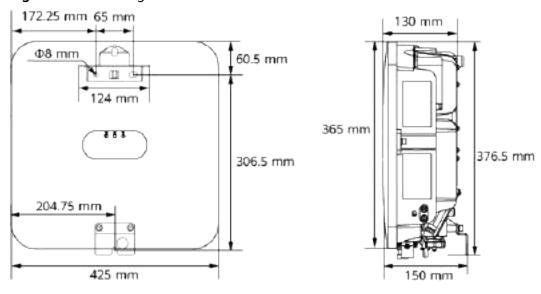
Figure 4-1 Mounting bracket dimensions
