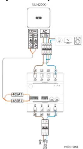
Figure 5-21 Connecting cables to the EMMA
