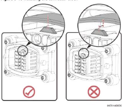
Figure 5-18 Installing the connector block
