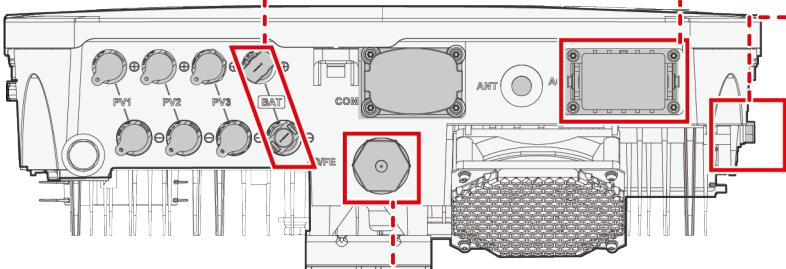
**EN-GB** Installing the Smart Dongle
