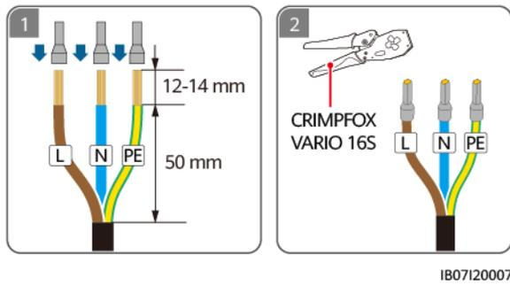
**Figure 5-11** Crimping SmartGuard-63A-AUS0 AC cord end terminals
