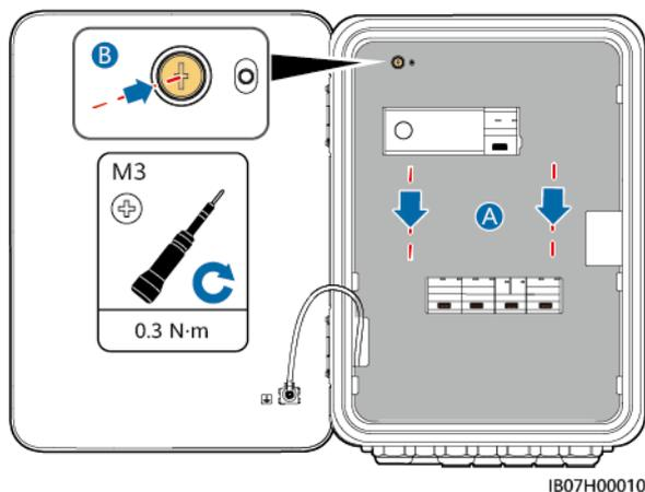
**Step 2** Before closing the maintenance compartment door, turn on the three switches shown in the following figure (using the connection to the LCO inverter as an example). During deployment and normal operation, do not operate the bypass switch shown in the figure.
