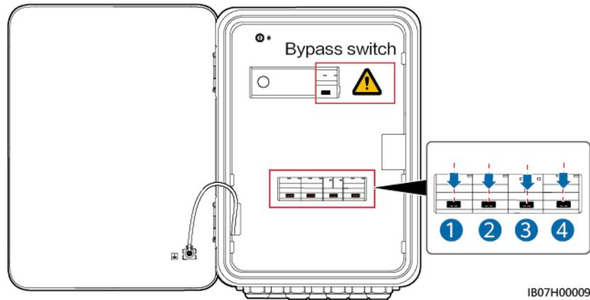
2. Remove the bypass switch latch, turn on the bypass switch, and then turn on switches ① and ④ shown in the figure.
