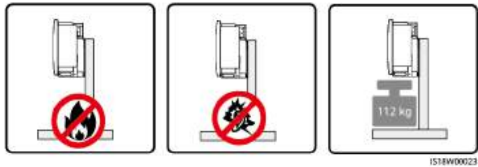
Figure 4-2 Mounting structure requirements
