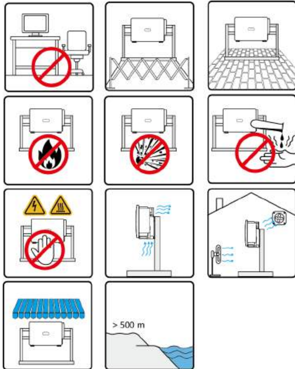
Figure 4-1 Installation environment requirements
