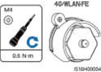
Figure 5-46 Installing anti-theft components for the Smart Dongle
