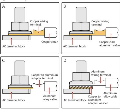
Figure D-1 Requirements for the OT/DT terminal
