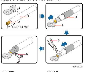
Figure D-2 Crimping an OT terminal
