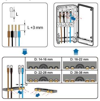
Figure 5-7 Single-core cable connection
