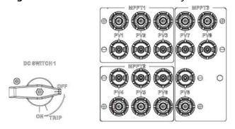
Figure 5-12 DC terminals controlled by DC SWITCH 2
