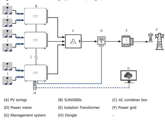
Figure 2-3 RS485 networking application (Dongle)
