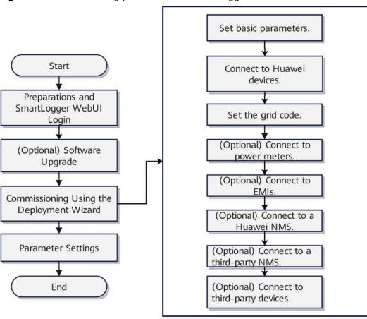
Figure 7-1 Commissioning process on the SmartLogger WebUI
