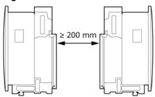
Figure 4-7 Stacked installation mode (not recommended)
