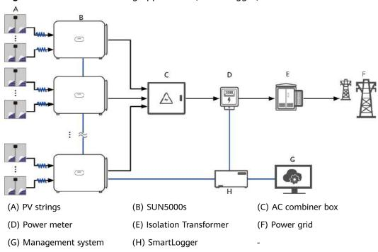
Figure 2-2 RS485 networking application (SmartLogger)
