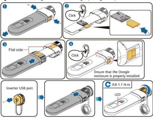
Figure 5-17 Installing the 4G Smart Dongle (SDongleB-06)
