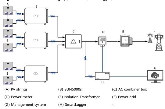
Figure 2-4 MBUS networking application (SmartLogger)
