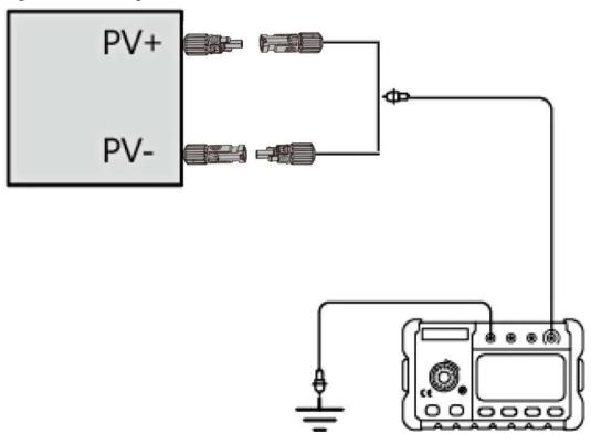
Figure 5-10 Testing the insulation resistance
