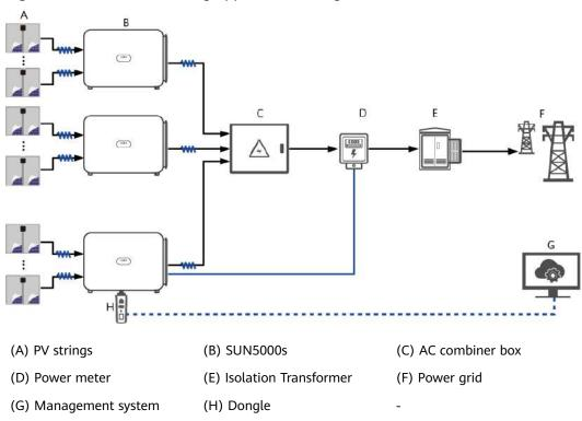
Figure 2-5 MBUS networking application (Dongle)
