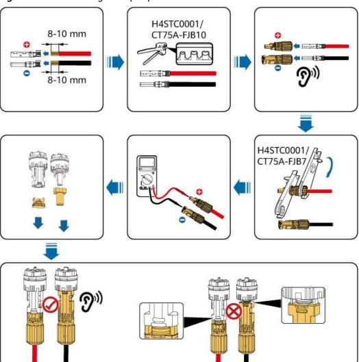
Figure 5-13 Connecting DC input power cables
